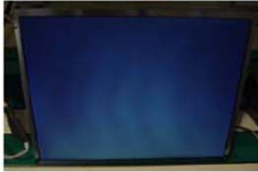
Panel Mura, Light leakage
